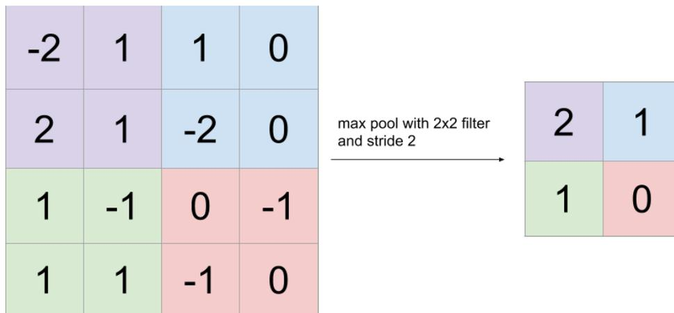
Fig. 10. Example of pooling operation using the max pooling with  $2 \times 2$  filter and stride 2. The maximum value of each  $2 \times 2$  colored square is selected for the output matrix in the position with the same color as the square.
